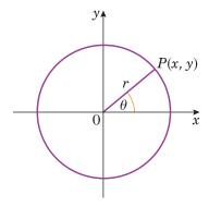
where (x, y) are the coordinates of the point P as it moves round the circumference of a circle with centre O and radius r, and OP makes an angle  $\theta$  with the +ve x-axis.
