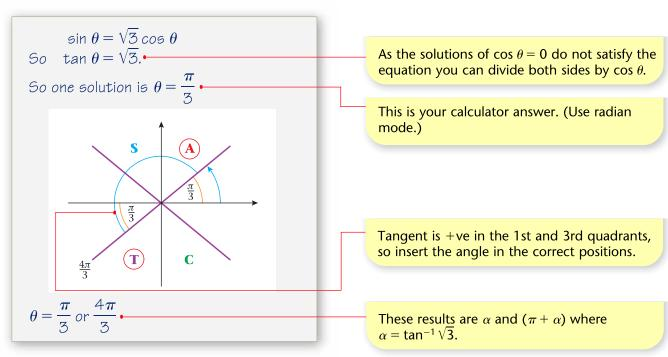
A first solution of the equation  $\tan x = k$  is your calculator value  $\alpha = \tan^{-1} k$ . A second solution is  $(180^{\circ} + \alpha)$ , or  $(\pi + \alpha)$  if you are working in radians. Other solutions are found by adding or subtracting multiples of 360° or  $2\pi$  radians.
