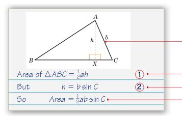
The perpendicular from A to BC is drawn and it meets BC at X. The length of AX = h.
