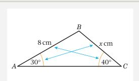
Always draw a diagram and carefully add the data. Here c = 8 (cm),  $C = 40^{\circ}$ ,  $A = 30^{\circ}$ , a = x (cm)
