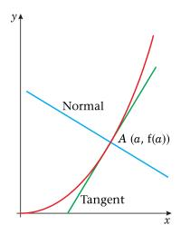
The gradient of the normal is  $-\frac{1}{f'(a)}$ , because the product of the gradients of lines which are at right angles is -1.
