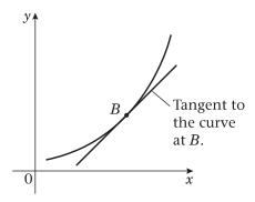
To find the gradient of the tangent at a point *B* on a curve with a known equation, you can find the gradient of chords joining *B* to other points close to *B* on the curve. You can then investigate the values of these gradients as the other points become closer to *B*. You should find the values become very close to a limiting value, which is the value of the gradient of the tangent, and is also the gradient of the curve at the point *B*.
