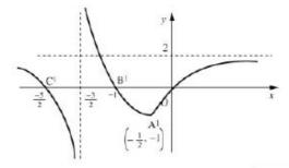
Stretch in the x direction with scale factor  $-\frac{1}{2}$  (or stretch in the x direction with scale factor  $\frac{1}{2}$  and reflect in the y-axis).
