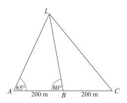
A landmark *L* is observed by a surveyor from three points *A*, *B* and *C* on a straight horizontal road, where AB = BC = 200 m. Angles *LAB* and *LBA* are 65° and 80° respectively (see diagram). Calculate
