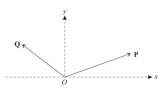
Two horizontal forces **P** and **Q** act at the origin *O* of rectangular coordinates Oxy (see diagram). The components of **P** in the *x*- and *y*-directions are 14 N and 5 N respectively. The components of **Q** in the *x*- and *y*-directions are -9 N and 7 N respectively.
