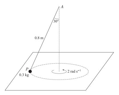
One end of a light inextensible string of length  $0.8 \,\mathrm{m}$  is attached to a fixed point A which lies above a smooth horizontal table. The other end of the string is attached to a particle P, of mass  $0.3 \,\mathrm{kg}$ , which moves in a horizontal circle on the table with constant angular speed  $2 \,\mathrm{rad} \,\mathrm{s}^{-1}$ . AP makes an angle of  $30^{\circ}$  with the vertical (see diagram).
