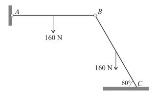
Two identical uniform rods, AB and BC, are freely jointed to each other at B, and A is freely jointed to a fixed point. The rods are in limiting equilibrium in a vertical plane, with C resting on a rough horizontal surface. AB is horizontal, and BC is inclined at  $60^{\circ}$  to the horizontal. The weight of each rod is  $160 \,\mathrm{N}$  (see diagram).
