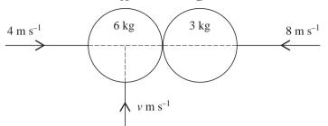
Two uniform smooth spheres A and B, of equal radius, have masses 6 kg and 3 kg respectively. They are moving on a horizontal surface when they collide. Immediately before the collision the velocity of A has components  $4 \text{ m s}^{-1}$  along the line of centres towards B, and  $v \text{ m s}^{-1}$  perpendicular to the line of centres. B is moving with speed  $8 \text{ m s}^{-1}$  along the line of centres towards A (see diagram). The coefficient of restitution between the spheres is *e*.
