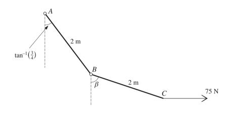
Two uniform rods *AB* and *BC*, each of length 2 m, are freely jointed at *B*. The weights of the rods are *W* N and 50 N respectively. The end *A* of *AB* is hinged at a fixed point. The rods *AB* and *BC* make angles  $\tan^{-1}\left(\frac{3}{4}\right)$  and  $\beta$  respectively with the downward vertical, and are held in equilibrium in a vertical plane by a horizontal force of magnitude 75 N acting at *C* (see diagram).
