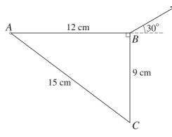
A uniform right-angled triangular lamina ABC with sides AB = 12 cm, BC = 9 cm and AC = 15 cm is freely suspended from a hinge at its vertex A. The lamina has mass 2 kg and is held in equilibrium with AB horizontal by means of a string attached to B. The string is at an angle of 30° to the horizontal (see diagram). Calculate the tension in the string. [4]
