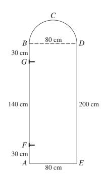
A door is modelled as a lamina *ABCDE* consisting of a uniform rectangular section *ABDE* of weight 60 N and a uniform semicircular section *BCD* of weight 10 N and radius 40 cm. *AB* is 200 cm and *AE* is 80 cm. The door is freely hinged at *F* and *G*, where *G* is 30 cm below *B* and *F* is 30 cm above *A* (see diagram).
