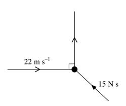
A ball of mass 0.5 kg is moving with speed  $22 \text{ m s}^{-1}$  in a straight line when it is struck by a bat. The impulse exerted by the bat has magnitude 15 N s and the ball is deflected through an angle of 90° (see diagram). Find
