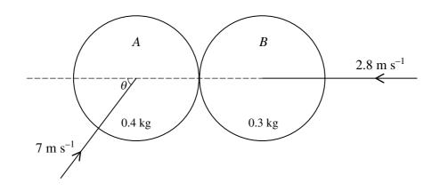
Two uniform smooth spheres A and B of equal radius are moving on a horizontal surface when they collide. A has mass 0.4 kg and B has mass 0.3 kg. Immediately before the collision A is moving with speed 7 m s<sup>-1</sup> at an acute angle  $\theta$  to the line of centres, where  $\cos \theta = 0.6$ , and B is moving with speed 2.8 m s<sup>-1</sup> along the line of centres (see diagram). The coefficient of restitution between the spheres is 0.7. Find
