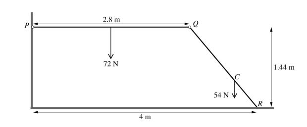
A uniform rod PQ has weight 72 N. A non-uniform rod QR has weight 54 N and its centre of mass is at C, where QC = 2CR. The rods are freely jointed to each other at Q. The rod PQ is freely jointed to a fixed point of a vertical wall at P and the rod QR rests on horizontal ground at R. The rod PQ is 2.8 m long and is horizontal. The point R is 1.44 m below the level of PQ and 4 m from the wall (see diagram).
