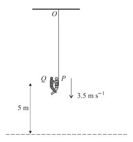
A circus performer P of mass 80 kg is suspended from a fixed point O by an elastic rope of natural length 5.25 m and modulus of elasticity 2058 N. P is in equilibrium at a point 5 m above a safety net. A second performer Q, also of mass 80 kg, falls freely under gravity from a point above P. P catches Q and together they begin to descend vertically with initial speed 3.5 m s<sup>-1</sup> (see diagram). The performers are modelled as particles.
