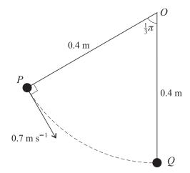
A particle P of mass 0.8 kg is attached to a fixed point O by a light inextensible string of length 0.4 m. A particle Q is suspended from O by an identical string. With the string OP taut and inclined at  $\frac{1}{3}\pi$  radians to the vertical, P is projected with speed 0.7 m s<sup>-1</sup> in a direction perpendicular to the string so as to strike Q directly (see diagram). The coefficient of restitution between P and Q is  $\frac{1}{7}$ .
