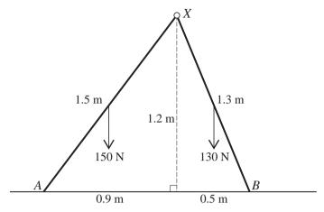
Two uniform rods XA and XB are freely jointed at X. The lengths of the rods are 1.5 m and 1.3 m respectively, and their weights are 150 N and 130 N respectively. The rods are in equilibrium in a vertical plane with A and B in contact with a rough horizontal surface. A and B are at distances horizontally from X of 0.9 m and 0.5 m respectively, and X is 1.2 m above the surface (see diagram).
