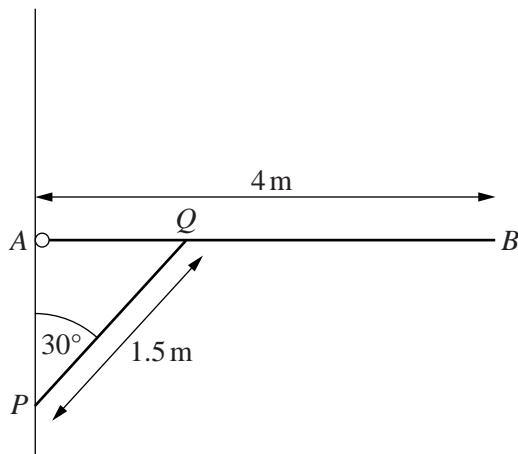
A uniform beam  $AB$  of mass  $15\text{ kg}$  and length  $4\text{ m}$  is freely hinged to a vertical wall at  $A$ . The beam is held in equilibrium in a horizontal position by a light rod  $PQ$  of length  $1.5\text{ m}$ .  $P$  is fixed to the wall vertically below  $A$  and  $PQ$  makes an angle of  $30^\circ$  with the vertical (see diagram). The force exerted on the beam at  $Q$  by the rod is in the direction  $PQ$ . Find
