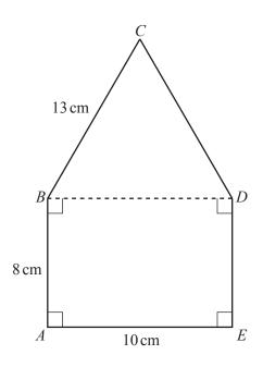
A uniform lamina *ABCDE* consists of a rectangle *ABDE* and an isosceles triangle *BCD* joined along their common edge. AB = DE = 8 cm, AE = BD = 10 cm and BC = CD = 13 cm (see diagram).
