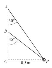
A small smooth ring *P* of mass 0.4 kg is threaded onto a light inextensible string fixed at *A* and *B* as shown in the diagram, with *A* vertically above *B*. The string is inclined to the vertical at angles of  $30^{\circ}$  and  $45^{\circ}$  at *A* and *B* respectively. *P* moves in a horizontal circle of radius 0.5 m about a point *C* vertically below *B*.
