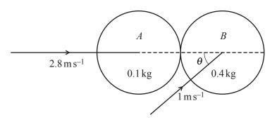
Two uniform smooth spheres A and B of equal radius are moving on a horizontal surface when they collide. A has mass 0.1 kg and B has mass 0.4 kg. Immediately before the collision A is moving with speed  $2.8 \text{ m s}^{-1}$  along the line of centres, and B is moving with speed  $1 \text{ m s}^{-1}$  at an angle  $\theta$  to the line of centres, where  $\cos \theta = 0.8$  (see diagram). Immediately after the collision A is stationary. Find
