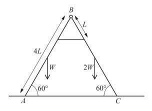
Two uniform rods AB and BC, each of length 4L, are freely jointed at B, and rest in a vertical plane with A and C on a smooth horizontal surface. The weight of AB is W and the weight of BC is 2W. The rods are joined by a horizontal light inextensible string fixed to each rod at a point distance L from B, so that each rod is inclined at an angle of  $60^{\circ}$  to the horizontal (see diagram).
