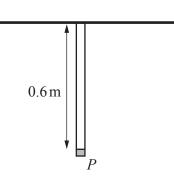
A small object P is attached to one end of each of two vertical light elastic strings. One string is of natural length 0.4 m and has modulus of elasticity 10 N; the other string is of natural length 0.5 m and has modulus of elasticity 12 N. The upper ends of both strings are attached to a fixed horizontal beam and P hangs in equilibrium 0.6 m below the beam (see diagram).
